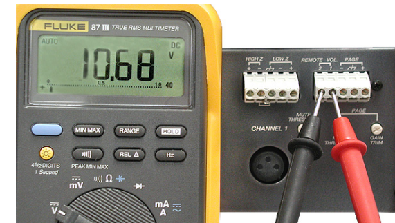
Measuring control voltage for a Peavey UMA™ 35T II: meter leads are oriented correctly
